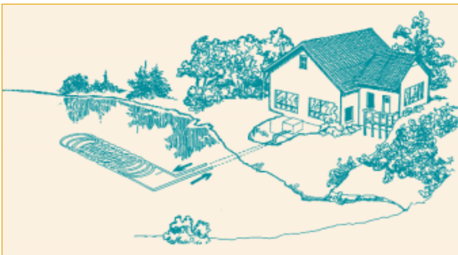
Lake loop systems (pond) can be used in either heating or cooling mode.
