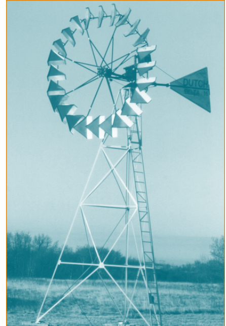
▲ Mechanical water pumping system.
