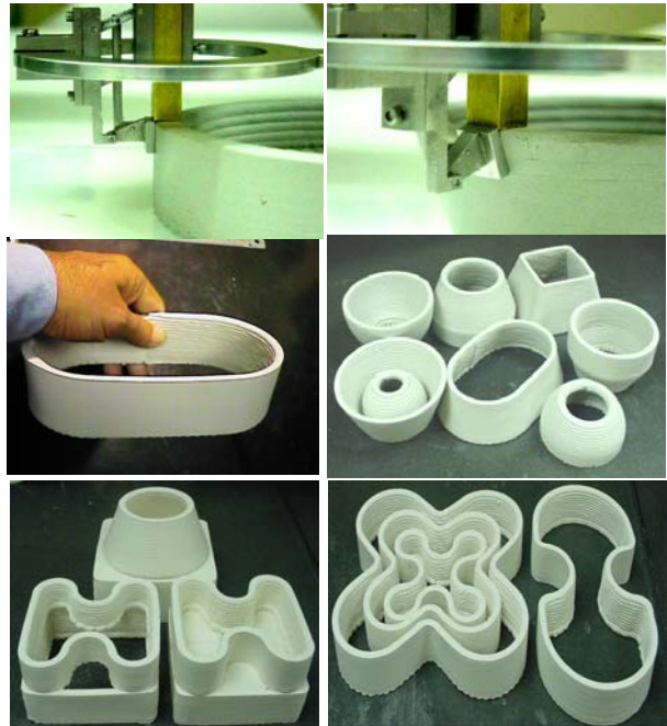
Figure 7. CC in operation and representative 2.5D and 3D shapes
